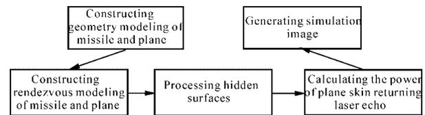
Fig.4 Flow chart of simulated laser imaging
