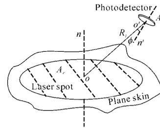
Fig.3 Relative position between receiving unit and laser spot
