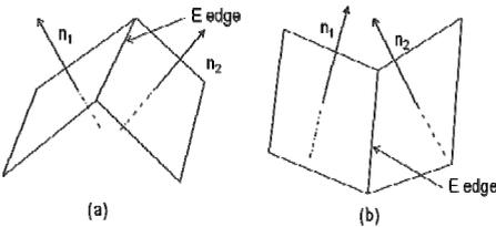
**Fig. 5.** The location relationship between two adjacent faces which make up of  $e$  edge. (a) Convex corner (b) Concave corner.
