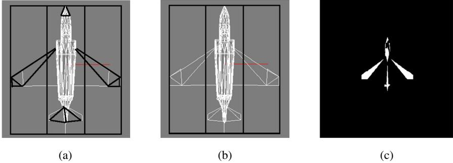
**Fig. 2.** Silhouette extraction algorithm. (a) The division of the projected image into several zones along Y-axis equally. (b) Fringe triangles representing the silhouette along Z-axis of projected image (not accurate). (c) Pruning result--3D silhouette of the model.
