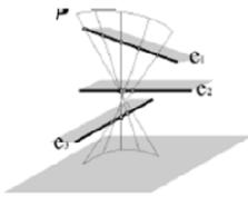
**Fig. 7.** The potential critical region induced in  $R^3$  by three edges  $e_1, e_2$  and  $e_3$  (excluding the region between the features) and (at the bottom of the diagram) its intersection with a portion of the sphere at infinity (From [5])
