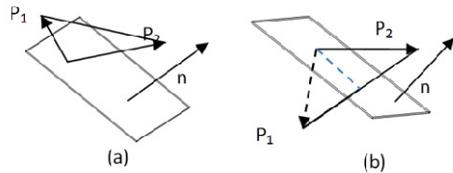
**Fig. 8.** Two vertexes of edge  $e_1$  and face  $n$ . (a) two vertexes are located in the same side of face (positive side). (b) two vertexes are located in the different sides of face.
