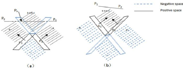
**Fig. 9.** Two vertexes of  $e_j$  and two faces adjacent to  $e_i$ . (a) Convex corner (b) Concave corner
