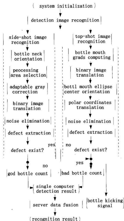
Fig.2. Detection system flow chart
